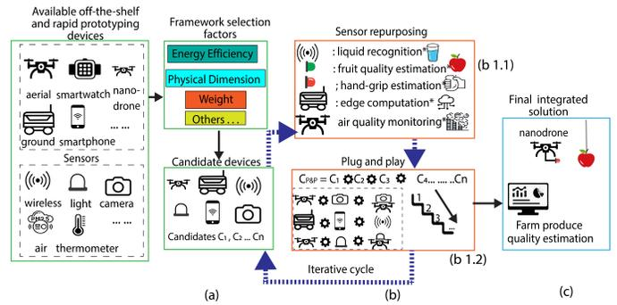
**Figure 2: Framework to re-purpose [25, 38, 47] and integrate [45] off-the-shelf components. (a) Off-the-shelf component selection (b) Re-purposing approach requiring 2 steps (c) Performance analysis of integrated solution**
