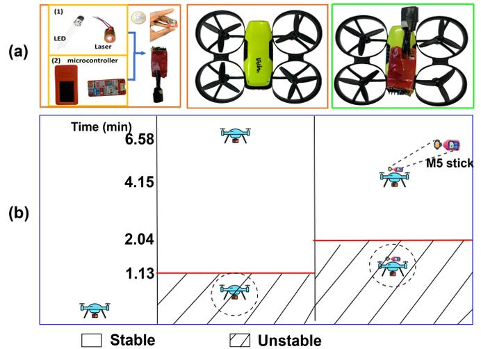
Figure 8: Nano-drone re-purposing; (a) Nano-drone and light sensor prototype; (b) Nano-drone operational flight time.
