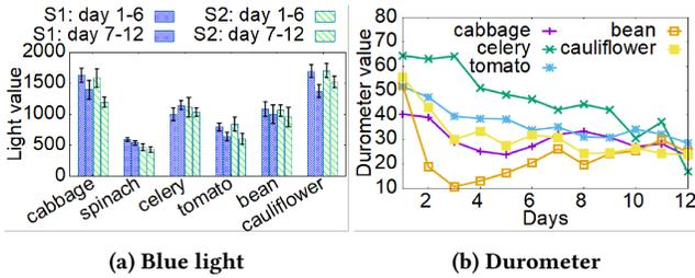
Figure 6: Light characterization for vegetable; (a) Two-stage median + SD light values (b) Average durometer readings
